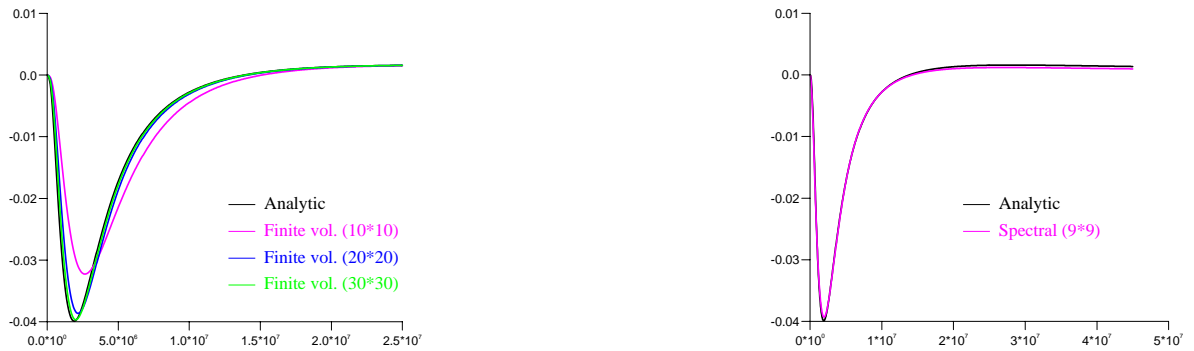
Figure 8: Values of the coupling term as functions of time at some point of the domain \Omega for various methods of calculating the coupling term
